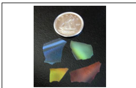
Figure 1. Photograph of chiral nematic mesoporous silica films (source: reference 3). The coin is for scale.
